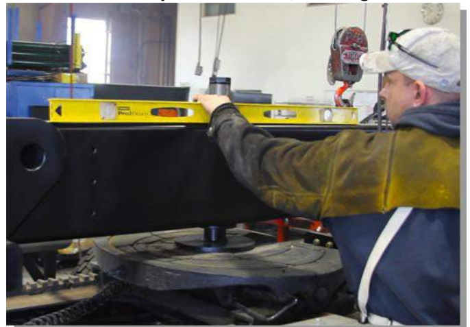
#6) Adjust height of kingpin, leveling beam on truck.
