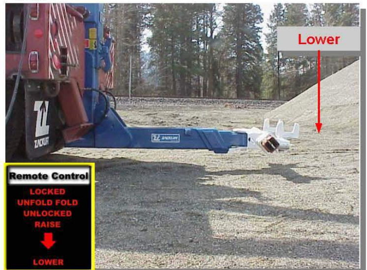
6) Lower Horizontal Tube until it is about 2" or 3" inches from the ground
