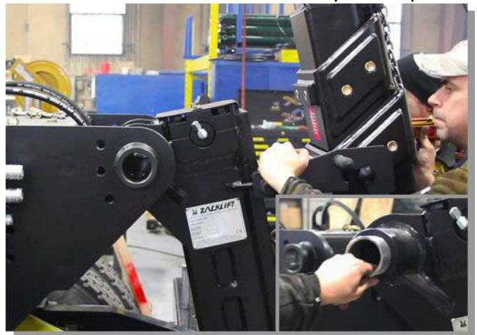
#18) Make sure the pivot bushing is inserted into the main pivot before installing Zacklift to subframe. See hydraulics section C-1 for connection instructions and diagram.
