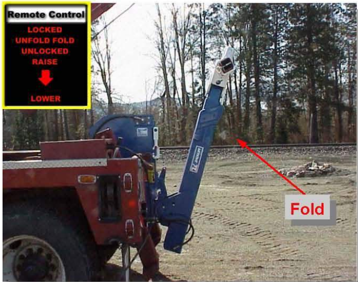
28) FOLD Horizontal Extend Tube for storage.
