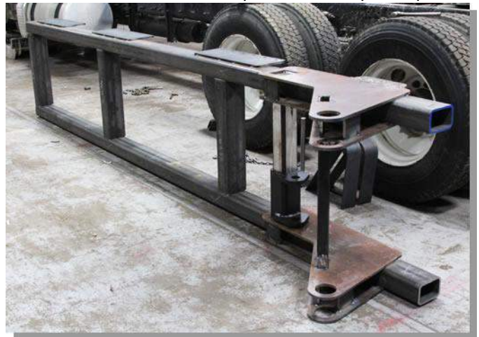
#16) Remove subframe from truck and fully weld all connections and placements. Then return subframe to truck and securely bolt in place.
