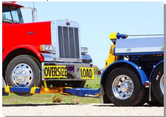
#10) Tilt up to get proper towing height.
