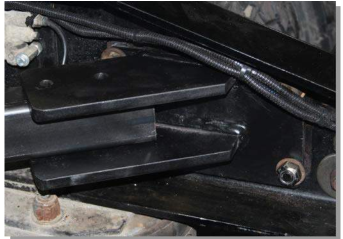
#4) Mount the fabricated mounting bracket loosely. Install Zacklift crossmember into brackets. Adjust as needed, then tighten bolts.
