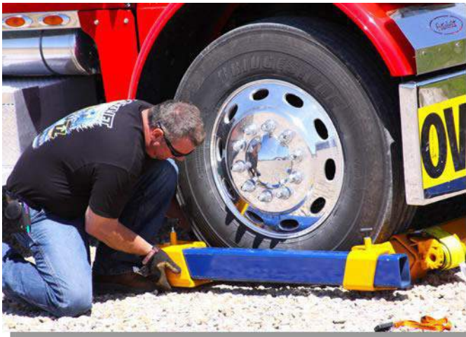
#7) Slide wheel tray onto wheel rod and against tire. Make sure pull pins are both fully engaged.
