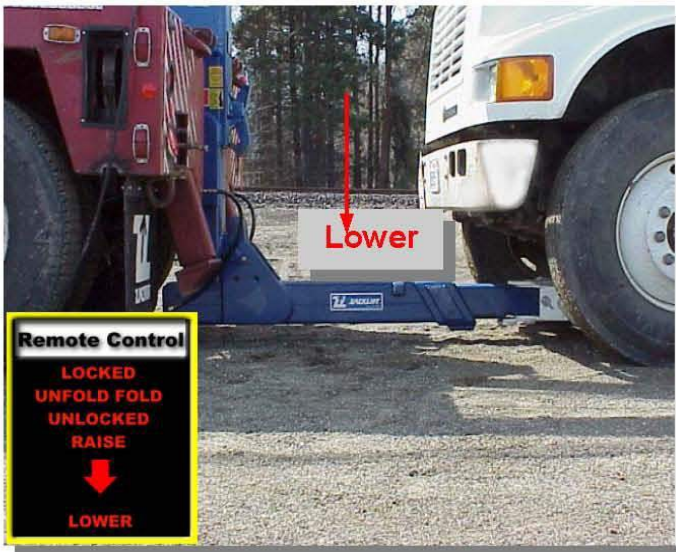
20) LOWER Horizontal Tube to within 2" - 3" from the ground.
