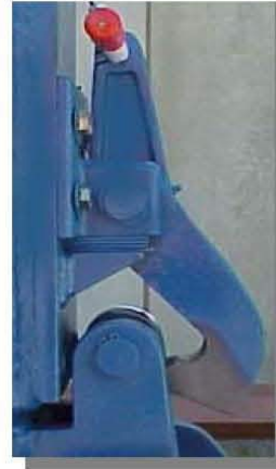
19) UNLOCK J Lock by pushing in towards main body.
