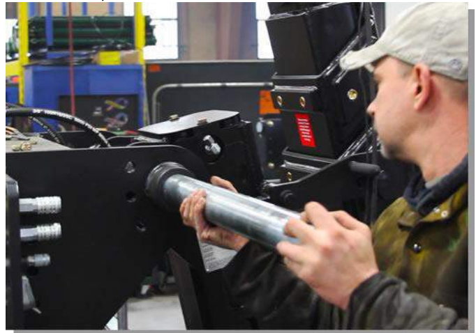
#16) Pin Zacklift into place with the pivot pin. Secure pivot pin with supplied bolts and lock nuts.
