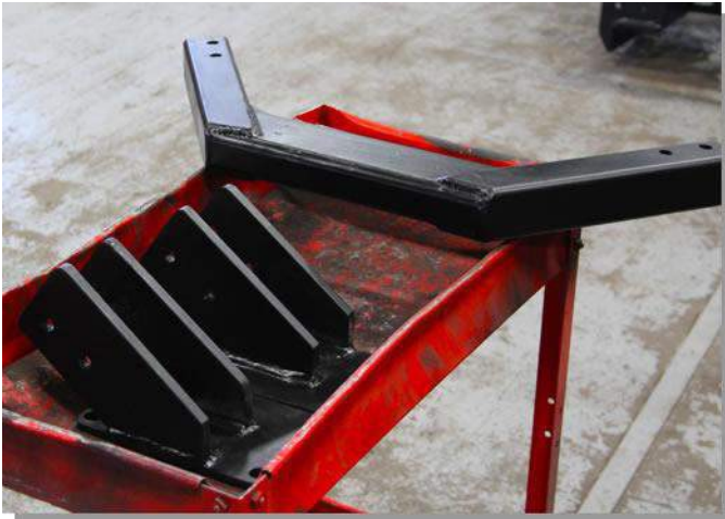
#3) Weld supplied ears to mounting plate so that crossmember slides in between ears. Mark hole locations from crossmember on ears and drill.
