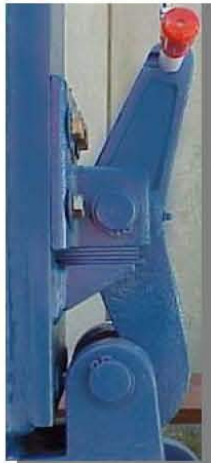
26) LOCK J Lock by pulling out & completely hooking around J Lock pin.
