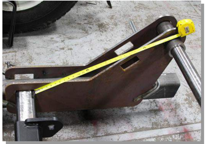
#14) The center of the pivot pin should be 30 inches from inner top corner of crossmember. Tack pivot bosses pin in place.
