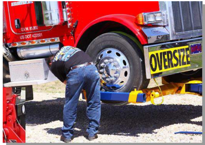
#8) Lift Zacklift fully into J-Lock. Pull strap over wheel and place hook into slot in rear of wheel tray.
