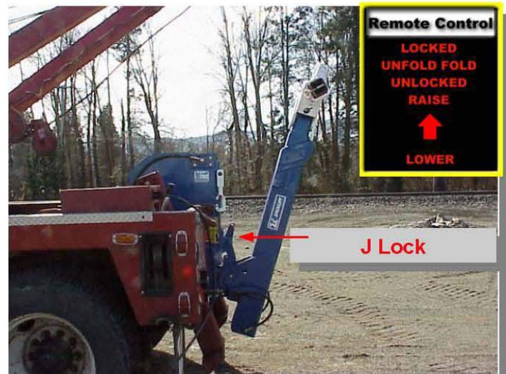
4) UNFOLD: CAUTION — do not unlock J Lock when unit is folded. Unlocking when unit is folded could result in injury or death.
