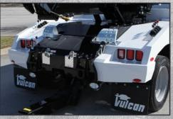
Vulcan light-duty conventional units come standard with tailboard D-Rings, wheel retainer storage pockets and separate boom and wheel lift controls for more versatility and ease of use.
