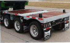
Steel Frame Wood Decks, Hydraulic Flip Third Axle - Optional Equipment
