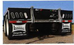
• 3 Stop Tail Turn with White Strobe LED Lights, Frame Prepped for Flip Third Axle - Standard
