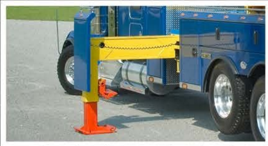
Standard top beam front outriggers with 212-inch stance
