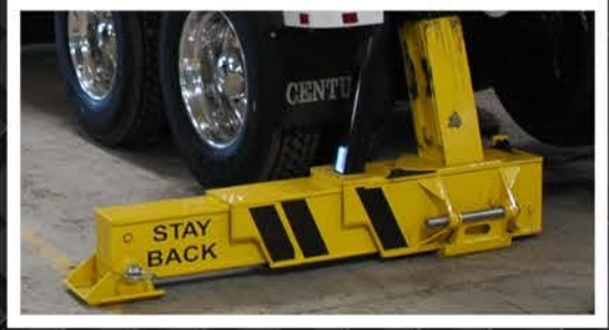
Standard three-stage rear outriggers with 174-inch stance
