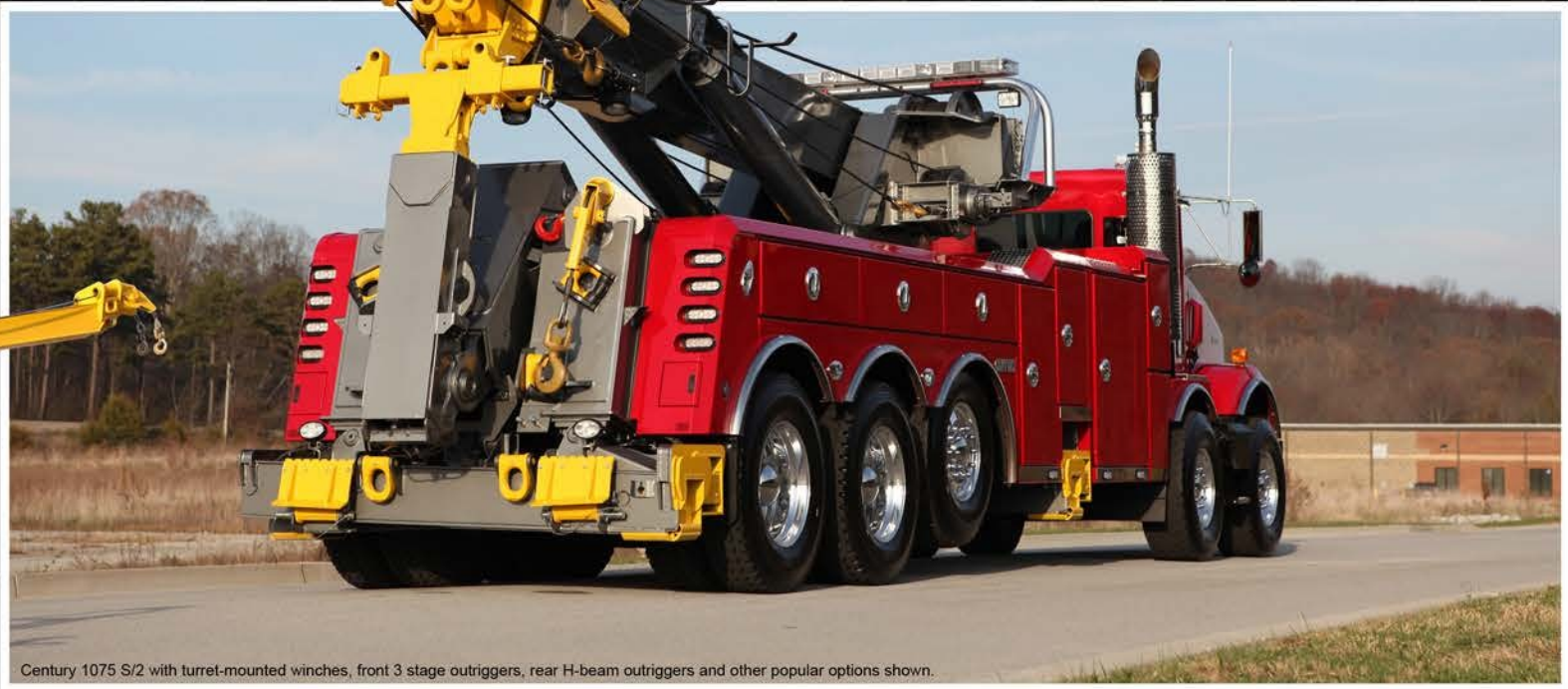
Century 1075 S/2 with turret-mounted winches, front 3 stage outriggers, rear H-beam outriggers and other popular options shown.
