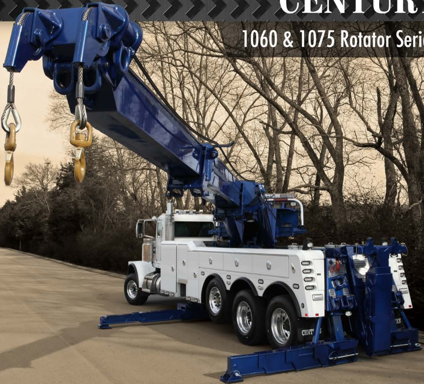
Century 1075 S with front 3 stage outriggers, rear 4 stage outriggers and other popular options shown.
