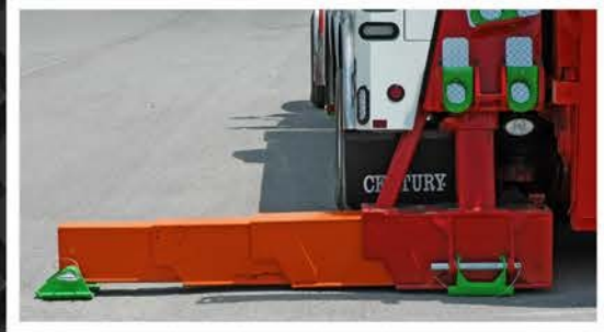
Optional four-stage rear outriggers with 220-inch stance
