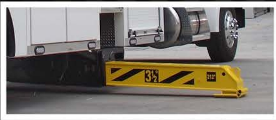
Optional two-stage front under-frame H-Beam outriggers with 212-inch stance
