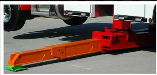
Optional three-stage front under-frame H-Beam outriggers with 262-inch stance
