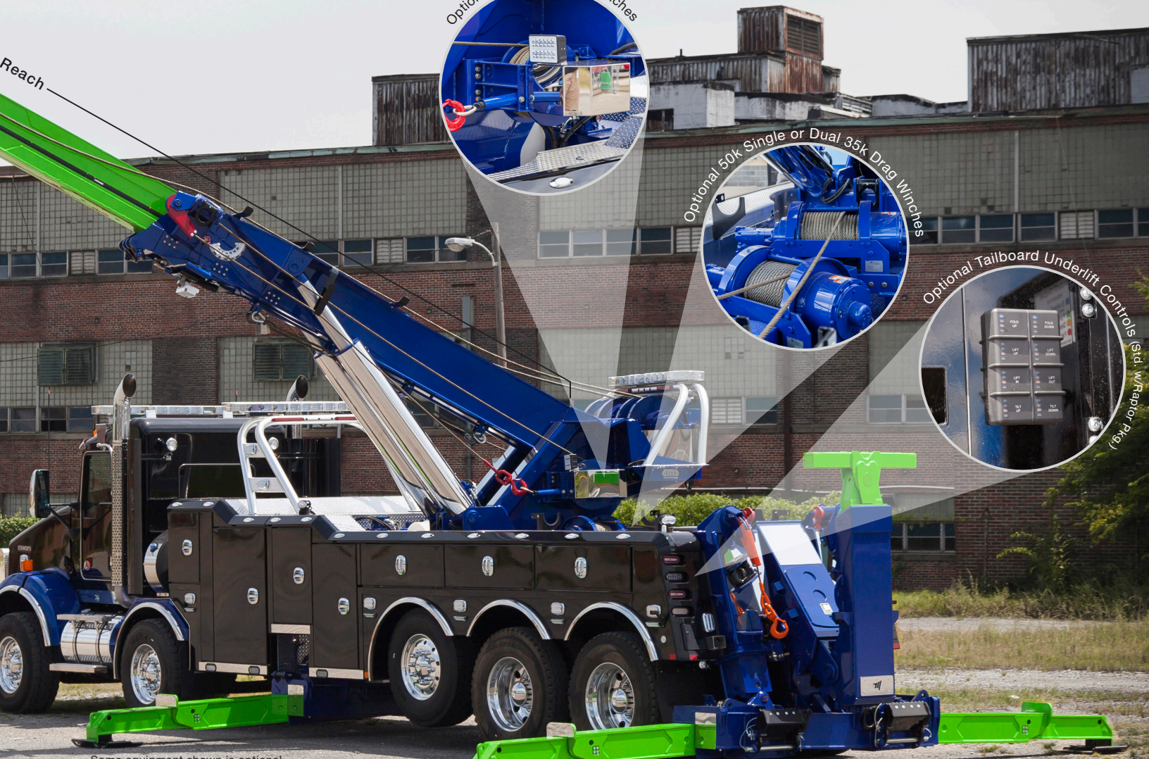
Optional H-Beam Outrigger with 262" Stance
