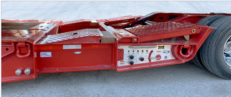
4 Position Extendable Lower Deck – Closed, 2½', 5', or 8' Lock Positions, Soft Transitions from Front Approach to Rear Bumper, Ramp Filler with Adjustable Slope Ramp for Safe Transition to Trunnion
