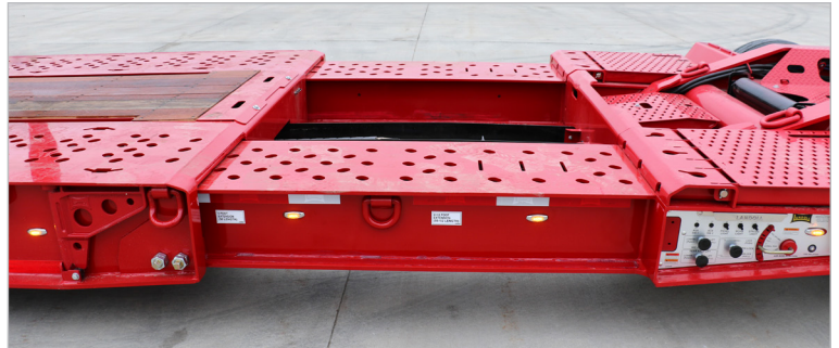
4 Position Extendable Lower Deck – Closed, 2½', 5', or 8' Lock Positions, Soft Transitions from Front Approach to Rear Bumper, Ramp Filler with Adjustable Slope Ramp for Safe Transition to Trunnion
