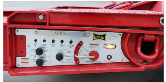
Rear Mounted Control Panel for Enhanced Work Lights, Extendable Locks, Ride Height Controls
